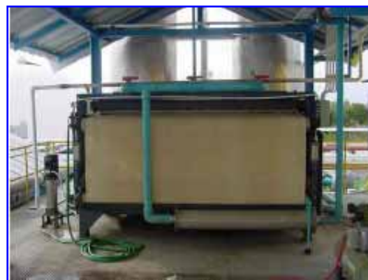
Dewatering Machine in Back-end Treatment Process
