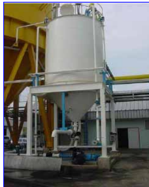
Feed Preparation Tank in HLAD Process
