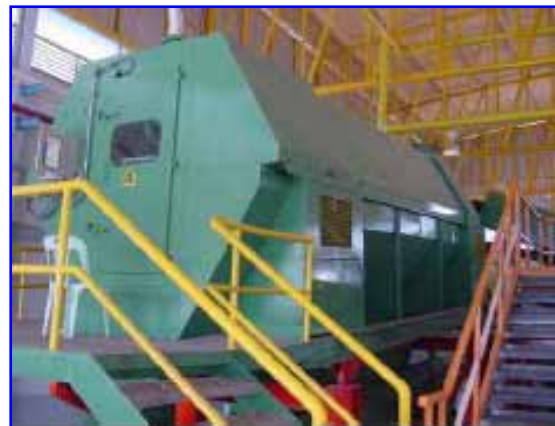
Drum Screen M/C in FET process
