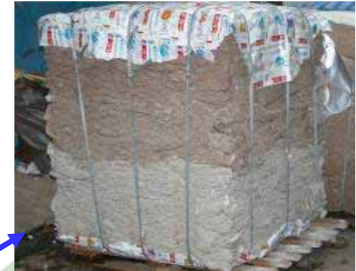
Pulp recovered from hydropulping
