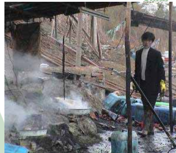
Chemical stripping operation (computer chips)
