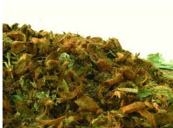
Coconut-shell biofilter at the Phitsanulok MBPT facility
