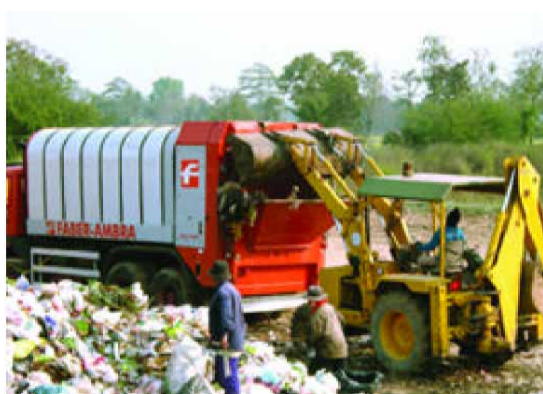
Homogenizing drum at work in Phitsanulok
