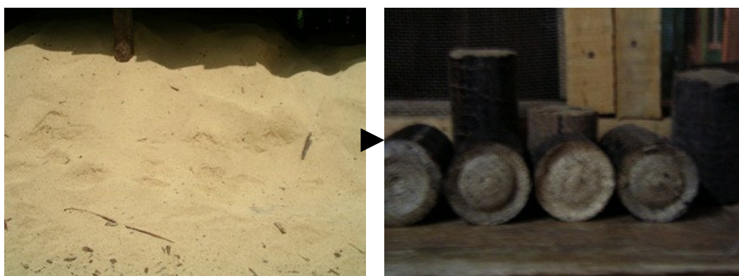
Sawdust to briquette for reuse as firewood
