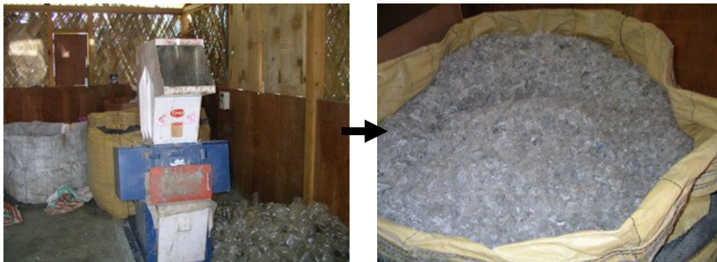
PET bottles to pellets for reducing bulk in transportation, storage and higher price
