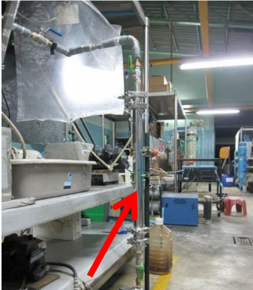
Monolith Ceramic Micro filter membrane with 0.1\ \mu\text{m} pore size
