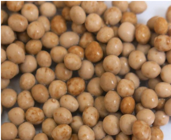
Matured PVA-gel (Settling velocity 228 m/h with biomass attachment of 0.5gVSS/gPVA-gel)
