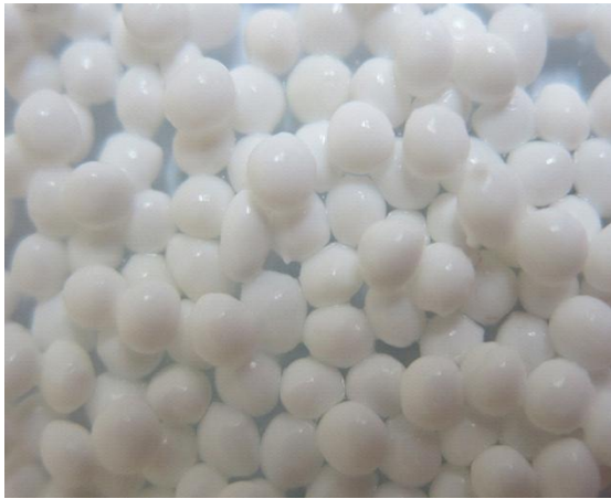
New PVA-gel (Settling velocity 143 m/h)
