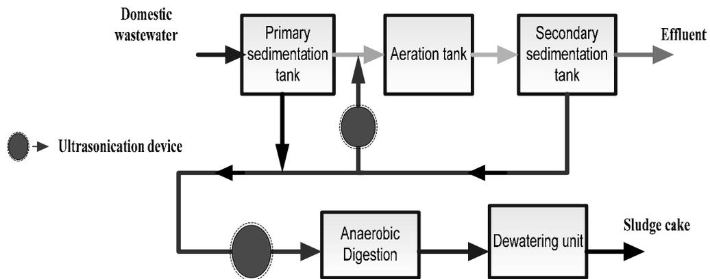
Figure 2.6 Location of ultrasonication in the sludge treatment
