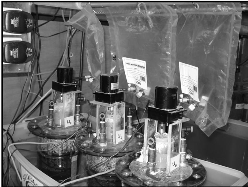
A7: Mixer, Air seal and Teflon biogas bag in Anaerobic digester experimental setup
