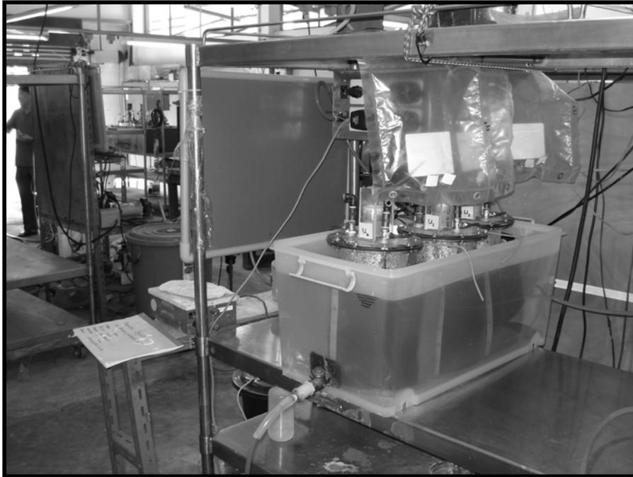
A6: Anaerobic digester experimental setup
