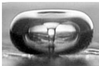
Figure 2.3 Cavitation Bubble
