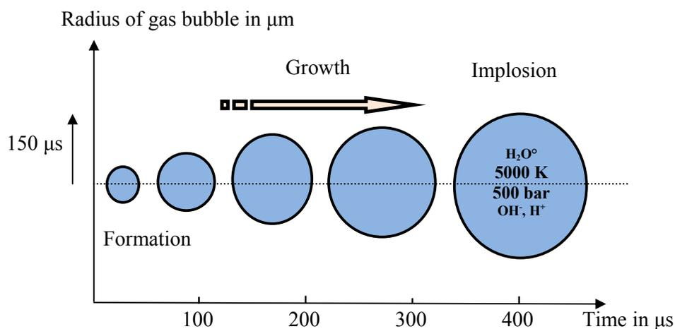
Figure 2.2 The illustration shows how a cavity builds up successively until it implodes
