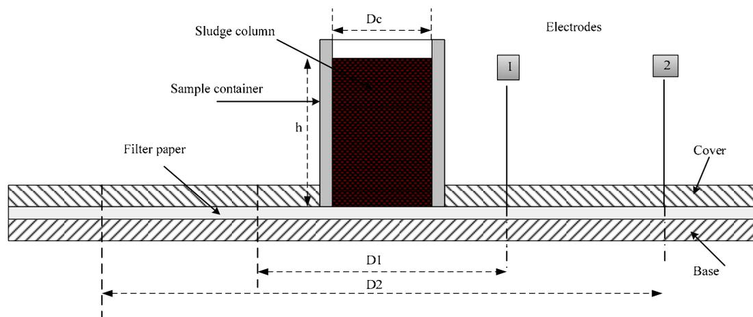
Figure 3.9 Schematic representation of CST apparatus
