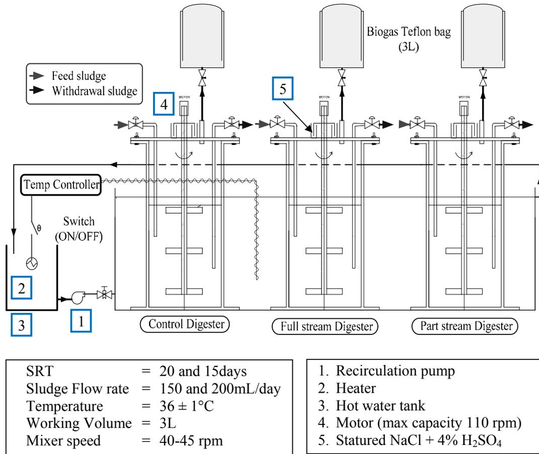
Figure 3.8 Experimental setup for anaerobic reactors used in this experiment
