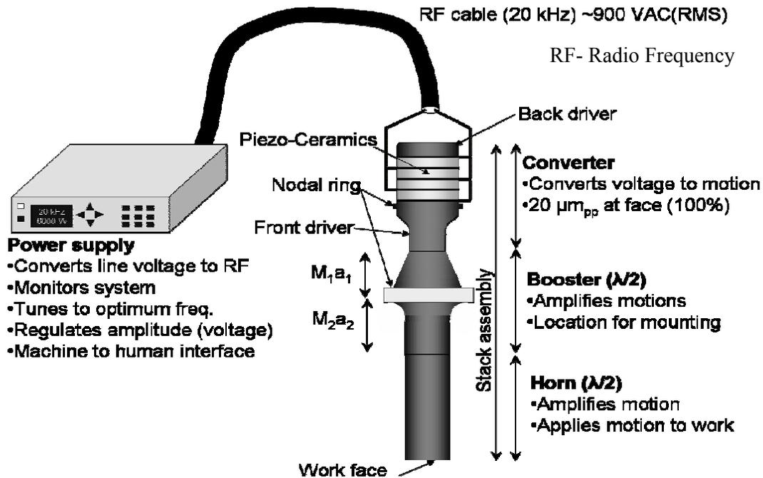
Figure 2.4 Details of typical 20 kHz piezo-electric ultrasonic system
