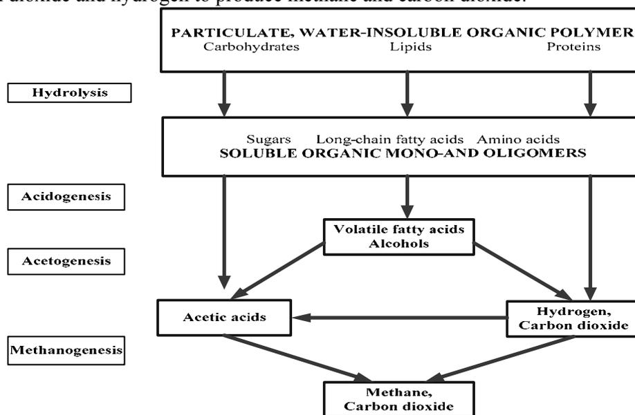
Figure 2.1 Summary of the anaerobic digestion chain
