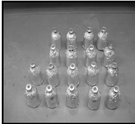
Figure 3.6 The serum bottle with capped with butyl rubber stopper used in BMP test
