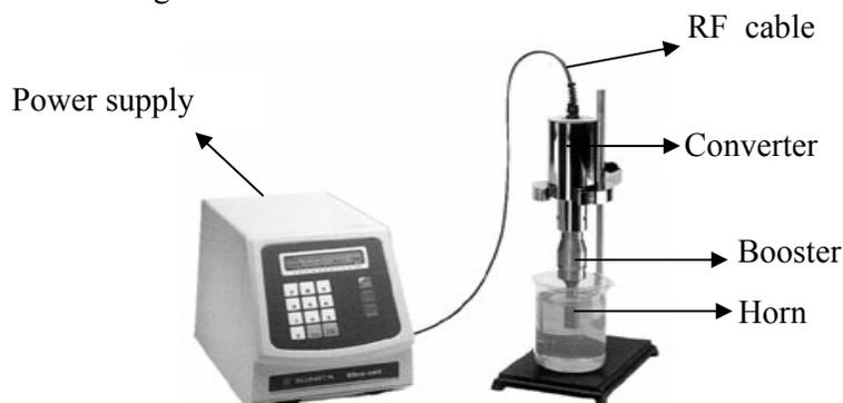
Figure 3.3 Ultrasonic equipment
