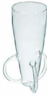
Figure 3.4a Rosett cooling cell
