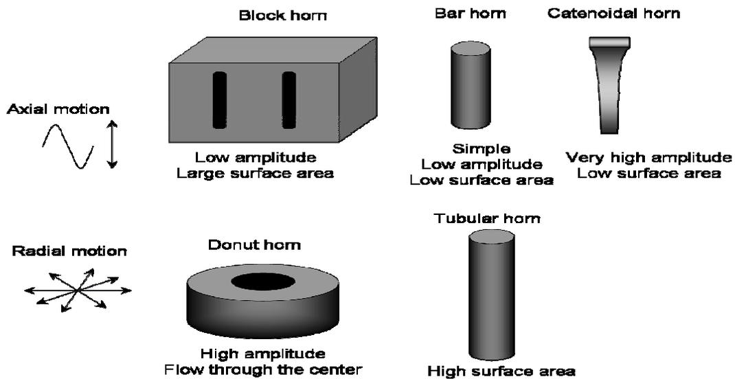
Figure 2.5 Examples of common horns used for liquid processing
