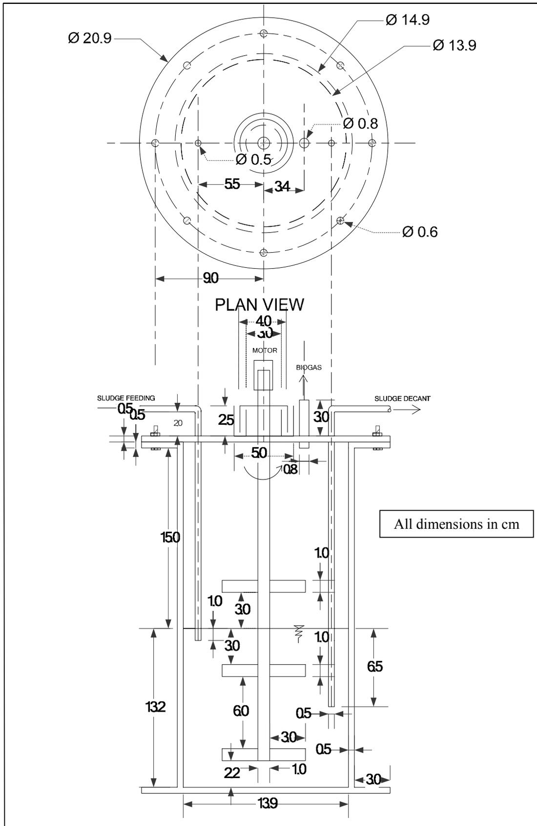
Figure 3.7 Anaerobic Digester Design
