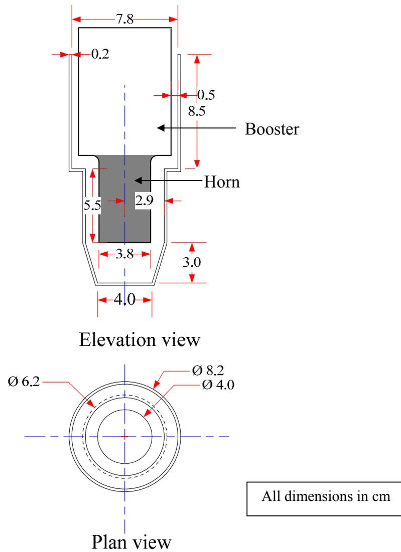
Figure 3. 5 Sonication chamber design with large horn and setup
