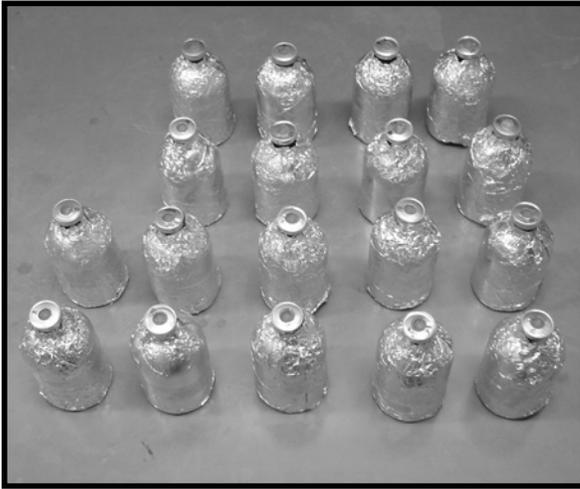
A2: BMP test experimental setup
