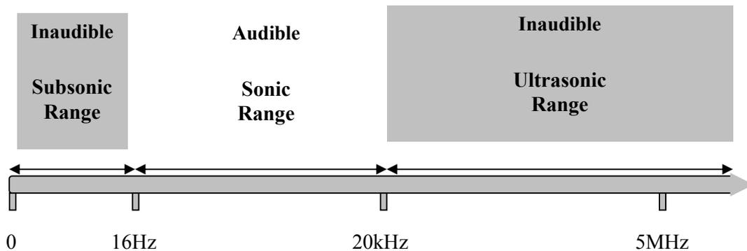
Ultrasound is above the human audible range, part of the sonic spectrum that ranges from 20 kHz to 10 MHz, is generated by a transducer in the Ultrasonic device that converts mechanical or electrical energy into high frequency acoustical (sound) energy. The sound energy is then fed to a horn that transmits the energy as high frequency vibrations to the liquid being processed. A wave propagates in a liquid through alternating cycles of compression and rarefaction.
