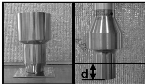
Figure 4.2 Large horn and large sonication chamber
