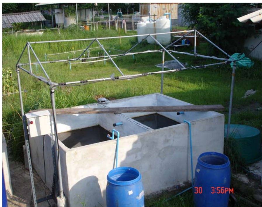
Figure C-2 Storage and evaporation tanks for Open Cell No.2 and 3 (During rainy season)
