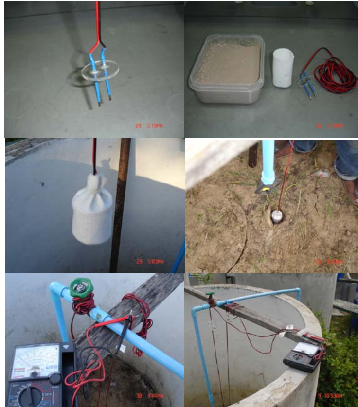
Figure C-5 Electrical resistance moisture content sensors and its using
