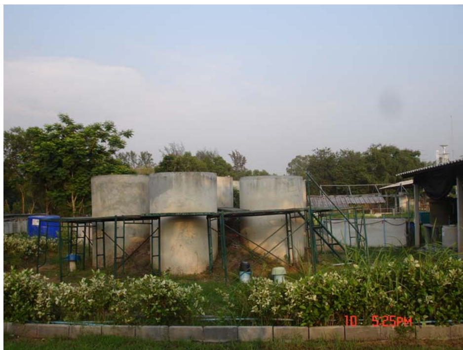
Figure C-1 Landfill lysimeters set up at Environmental Research Station of AIT
