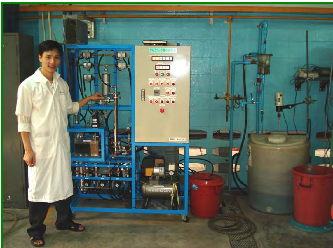
Figure A.1 The hybrid ceramic micro-filtration systems
