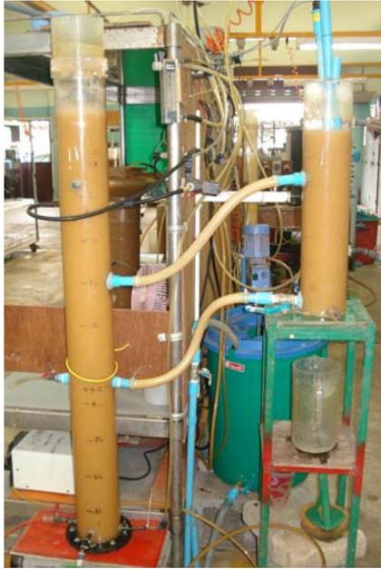
Figure A-14 Experimental setup of the continuous granulation MBR (CG-MBR) at AIT
