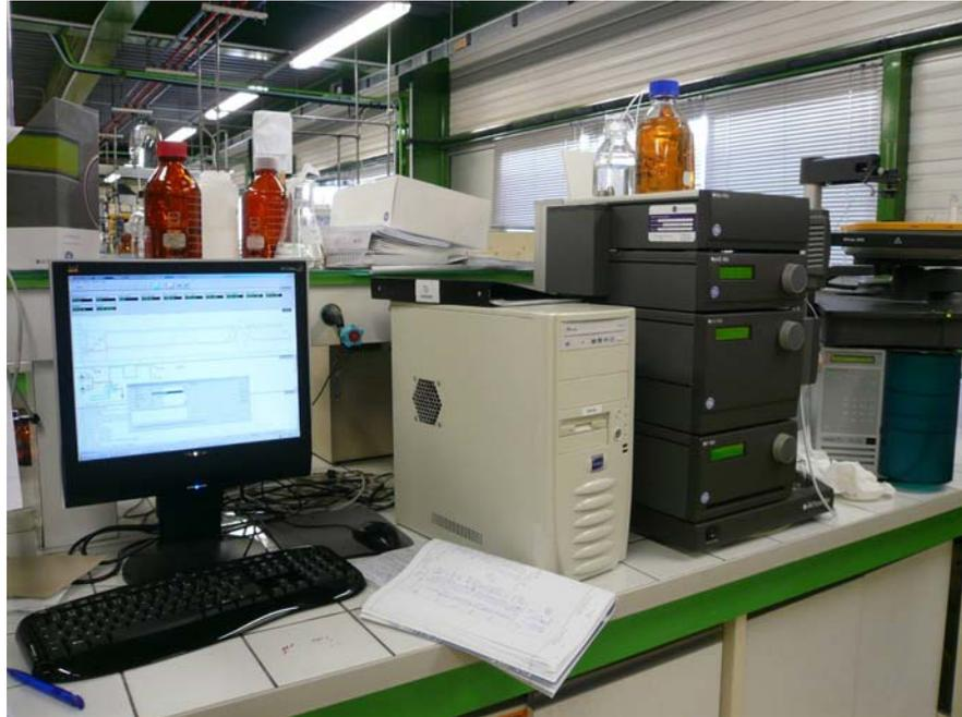
Figure A-12 HPLC system for size exclusion and hydrophobic interaction chromatography at INSA-Toulouse-France
