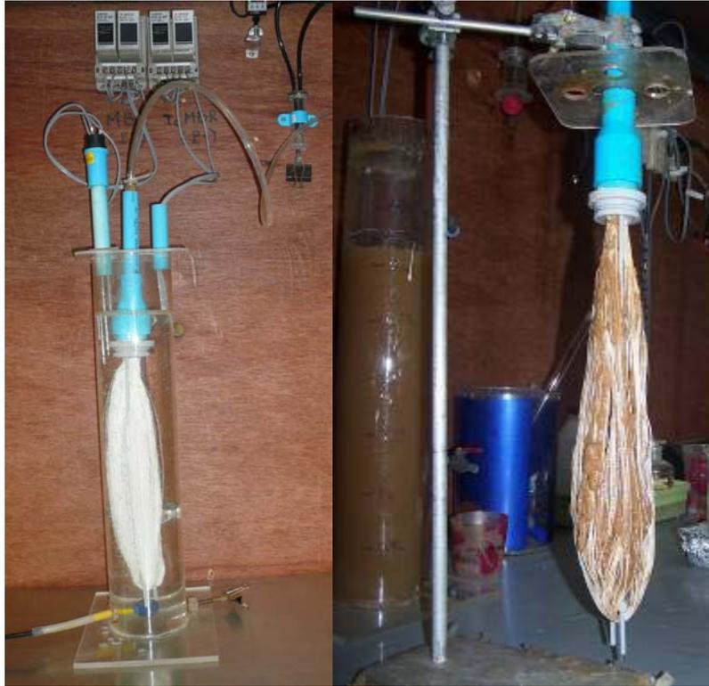
Figure A-4 Clean membrane (left) and fouled membrane (right) of the BG-MBR
