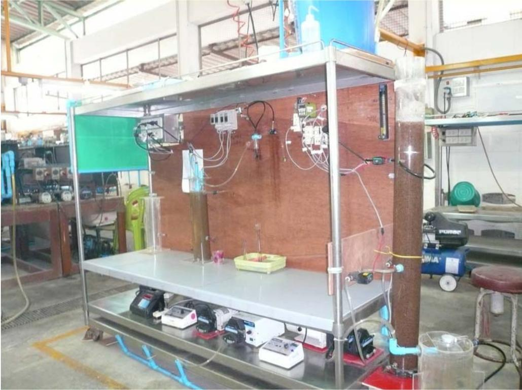
Figure A-1 Experimental set-up of the Batch Granulation MBR system (BG-MBR)
