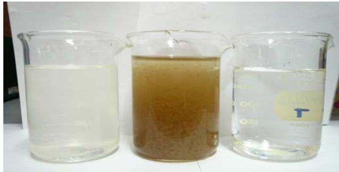
Figure A-2 From left to right (settler supernatant – MBR mixed liquor – membrane permeate)
