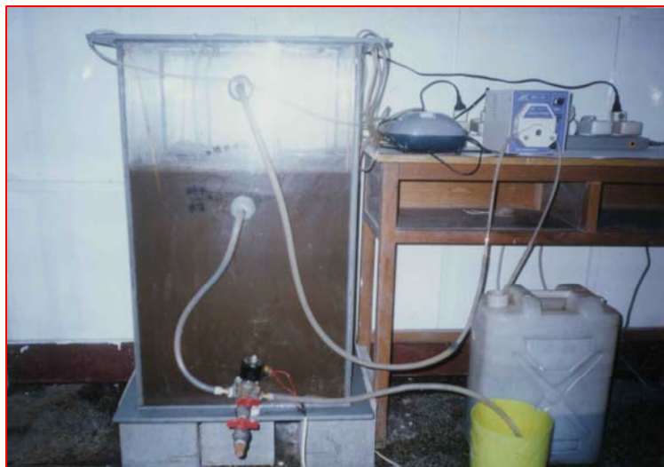
SBR Leachate treatment-China
