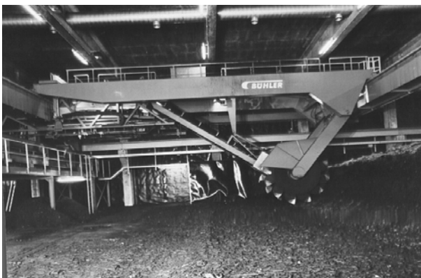
Figure 1: European and Asian composting systems. Left: Aerated pile composting in a rotting hall in Germany. Right: Windrow composting in Sri Lanka.
