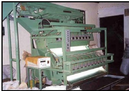
Color separating machine that electronically sorts the tea leaves into different grades
