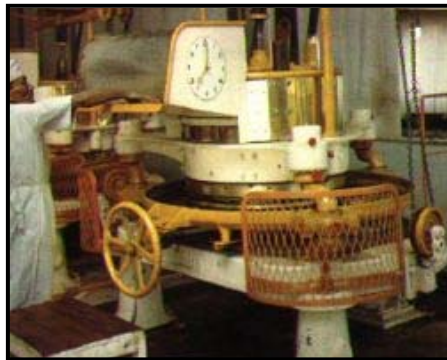
The Orthodox rolling machine twists the tea leaves to release its chemical compounds.
