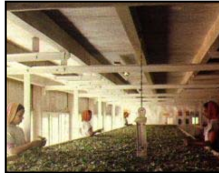
Withering troughs with a wet-dry bulb thermometer to monitor tea leaf moisture content
