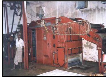
A conventional Endless Chain Pressure (ECP) dryer with continuously moving trays.
