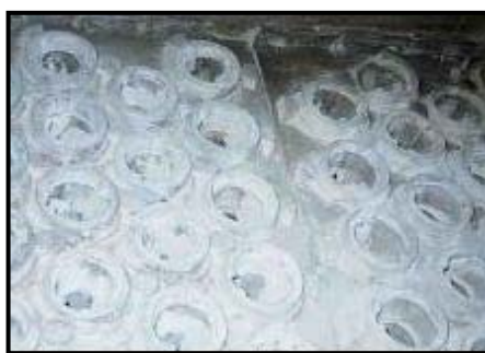
Blocked tubes of a wood-fired heater contributes to reduction in heat transfer efficiency
