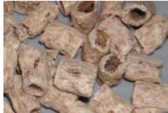
Cylindrical polypropylene (CP; inner Ø 3mm, outer Ø 4mm, length 5mm)
