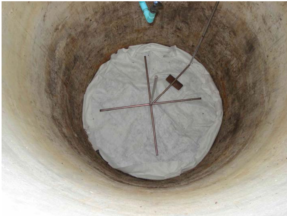
Figure B-2 Landfill lysimeter installation by Aeration & Leachate Recirculation systems
