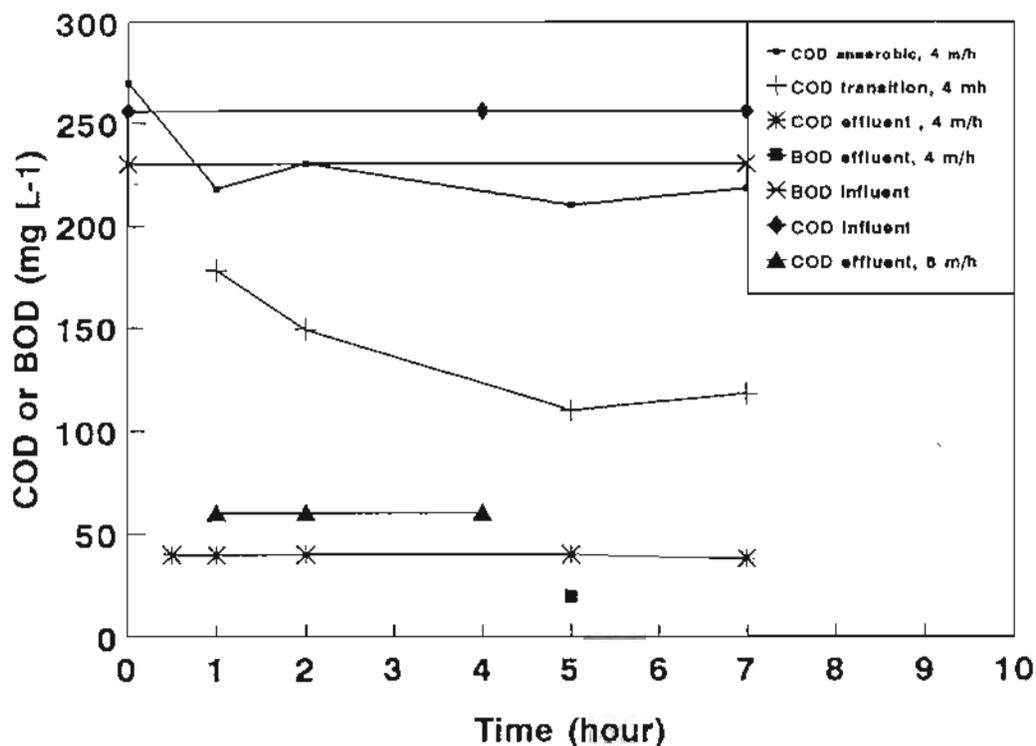
Figure 5. COD, BOD vs. time ( $T=30\text{ }^{\circ}\text{C}$ ,  $V=4\text{ m h}^{-1}$  &  $8\text{ m h}^{-1}$ ).
