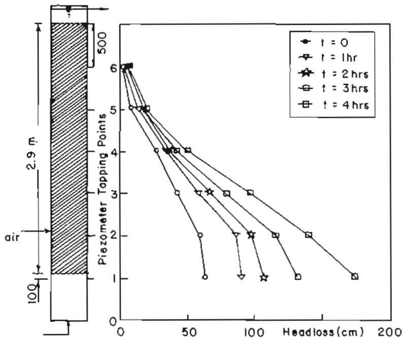
Figure 4b. Headloss profiles vs. time (filtration velocity =  $8 \text{ m h}^{-1}$ ,  $T=30 \text{ }^\circ\text{C}$ ).
