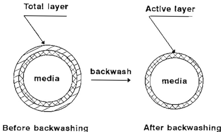
Figure 10. Fixed biomass before and after backwashing.
