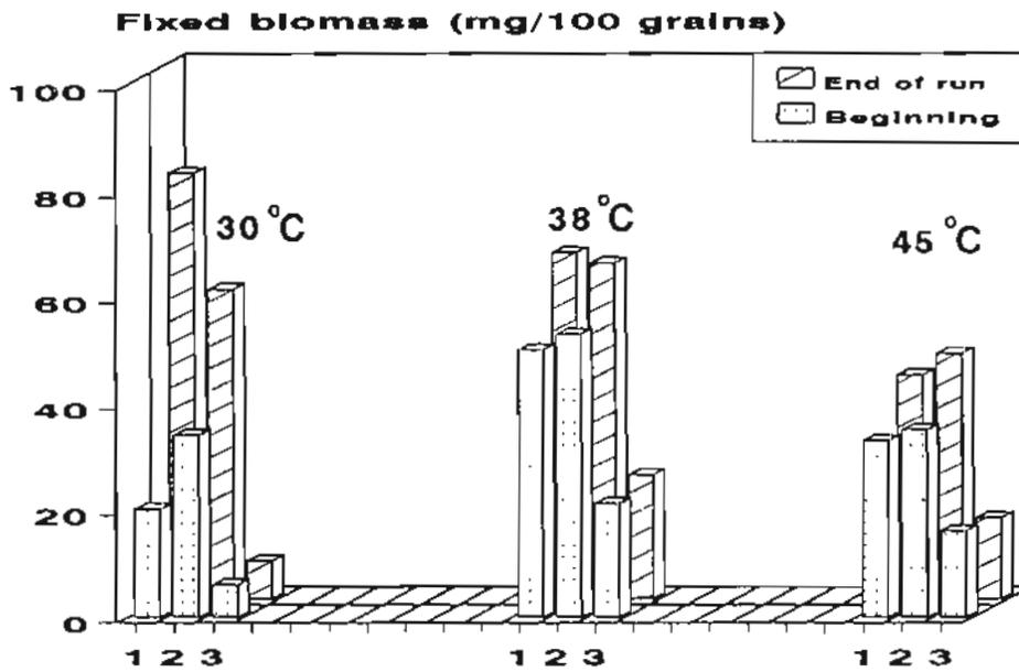
Figure 7. Fixed biomass vs. temperature (at filtration velocity  $2 \text{ m h}^{-1}$ , 1=anaerobic zone, 2=transition zone, 3=aerobic zone)
