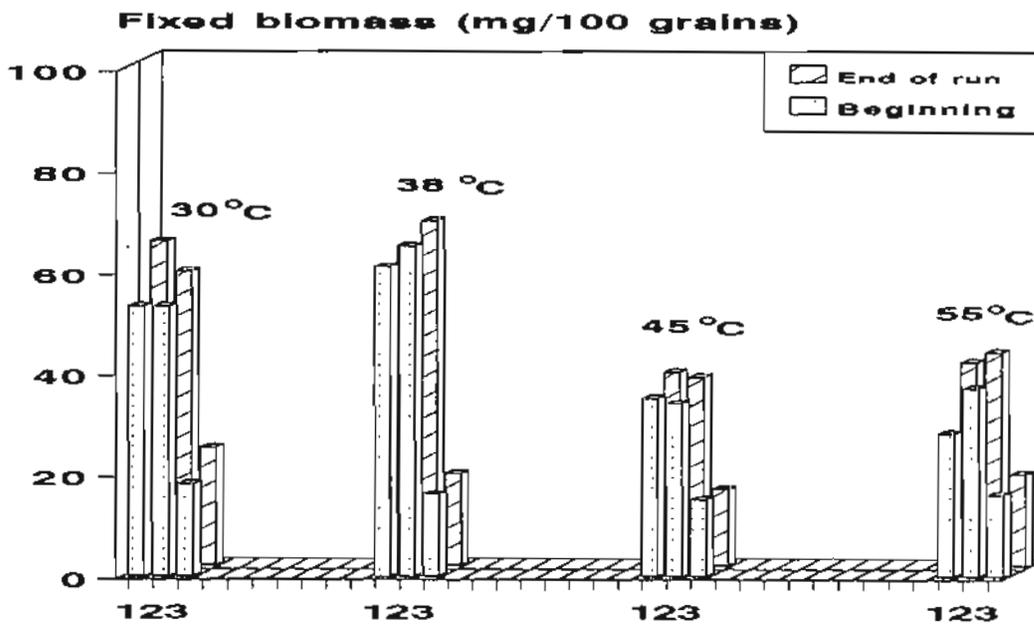
Figure 8. Fixed biomass vs. temperature (at filtration velocity  $6 \text{ m h}^{-1}$ , 1=anaerobic zone, 2=transition zone, 3=aerobic zone).
