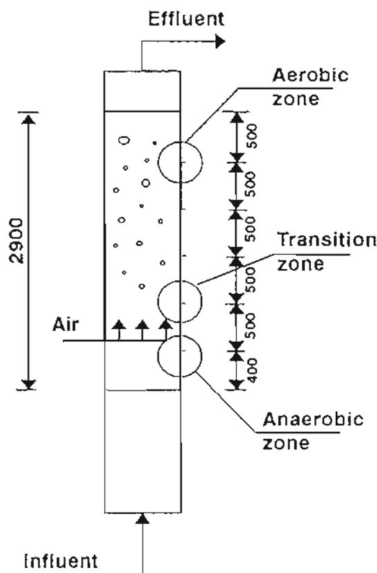
Figure 2. Sampling positions in the filter bed.
