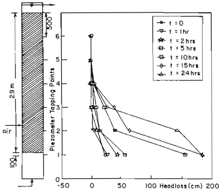
Figure 4a. Headloss profiles vs. time (filtration velocity =  $2 \text{ m h}^{-1}$ ,  $T=30 \text{ }^\circ\text{C}$ ).
