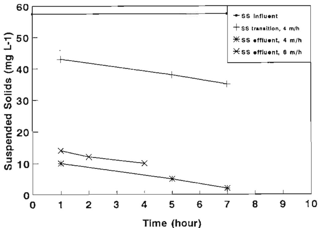
Figure 6. Suspended solids vs. time ( $T=30\text{ }^{\circ}\text{C}$ ,  $V=4\text{ m h}^{-1}$  &  $8\text{ m h}^{-1}$ ).
