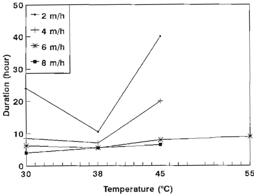
Figure 9. Filter run duration as a function of temperature and filtration velocities.
