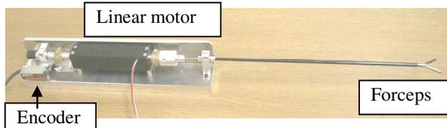
Fig. 10. Forceps connected to the Slave
