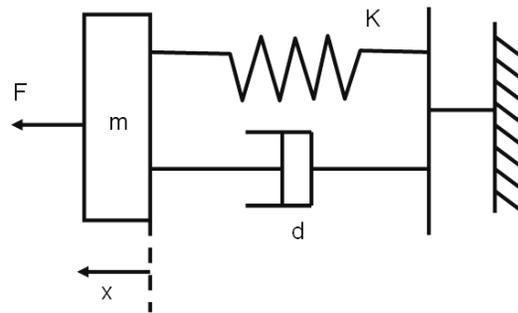
Fig.7. Virtual Spring Damper Model
