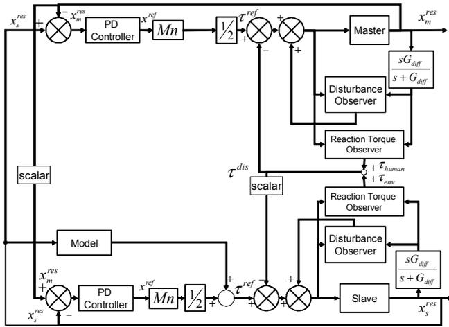
Fig. 9. Master model with Bilateral Control
