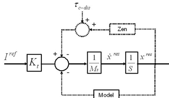
Fig. 8. Environment load and virtual model
